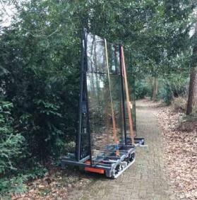
The TC1 carrier is the solution for horizontal transport of long, heavy construction material and equipment at a project site.
